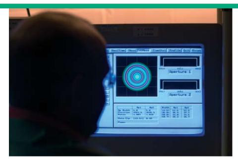
Fine-tuning of the violet laser beam profile gives the Luxel V-6 its outstanding hard dot characteristic for ultimate quality imaging (right). Precision engineering and alignment of the laser optics is the other half of the story (below).
