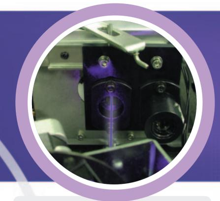
Fujifilm's laser pen boasts a life of over 5000 imaging hours — that's five years of typical use — giving large cost savings compared with multiple laser arrays used in thermal devices
