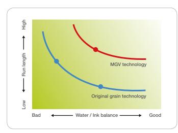
This diagram highlights how Fujifilm's MGV technology improves run lengths and ink/ water balance on press
