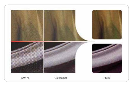
This diagram highlights the ability of PRO-T3 to reproduce various screening technologies and in particular 20µm FM.
