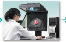
Two images are displayed on the two high-definition monitors. By wearing the polarized 3D glasses, a 3D image can be viewed through the half mirror.
