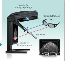
A stereoscopic image can be created instantly from two images, enabling immediate diagnosis after exposure. There is no need for complex image reconstruction or operations.
