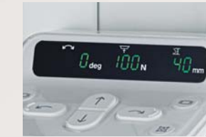
Shows swivel arm angle, compression force and breast thickness
