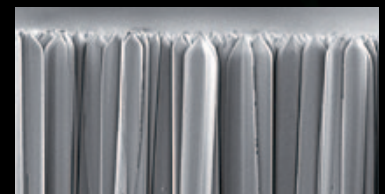
Crystal Structure of CsI
