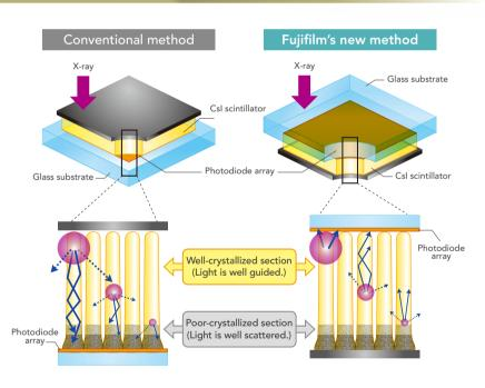
The novel type CsI:TI FPD, combining an adhesively coupled structure with ISS method, exhibits significant improvement in image quality than conventional CsI:TI FPDs and provides a way to reduce X-ray exposure to the patient.
